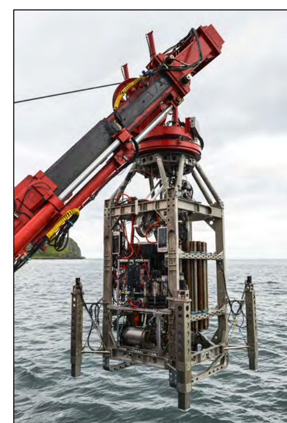
BGS British Geological Survey RD2 Rock Drill that will be used during WP3 to determine the permeability of chimney structures (image courtesy BGS).
